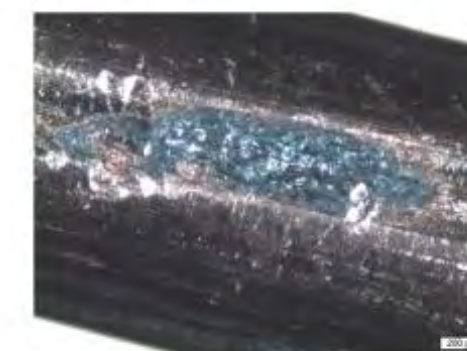
(b) Fretting on conductor wire surface
