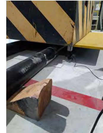
3 – Crush test for long term stacking
