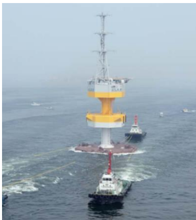
The 'Fukushima Kizuma' floating offshore substation project in Japan, rated at 25 MVA, (and right) FOSS being towed out to site (now decommissioned)
