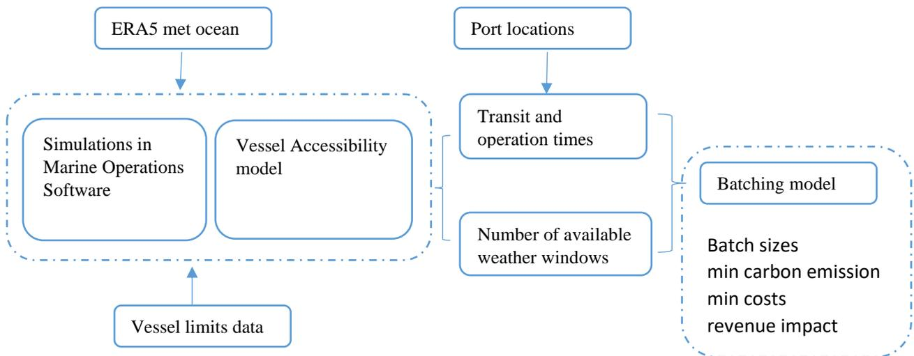
Figure 5.1: Model structure and process flow.
